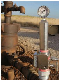
Charge the gas gun 150-300 psi above surface pressure on the well.
