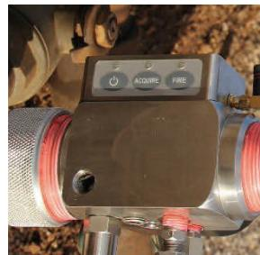
Press "Acquire" switch on gun and wait for the "Fire" light to stop blinking, then press "Fire" button when ready to shoot. Make sure the chamber pressure is greater than the well pressure.
